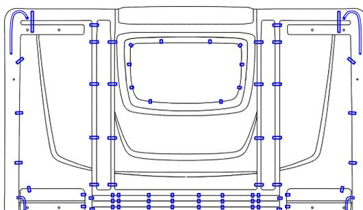
**Figure 11.** Adjusted CAD model of the truck rear panel optimized for a reduced bending and membrane springback.
