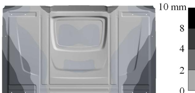
**Figure 3.** Truck rear panel with the calculated bending springback.
