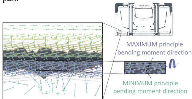
**Figure 7.** Principal bending moment within the resulting design proposal in a selected area of the part.
