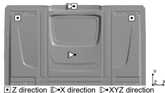
**Figure 2.** Boundary conditions to fix translational and rotational degrees of freedom during simulation.
