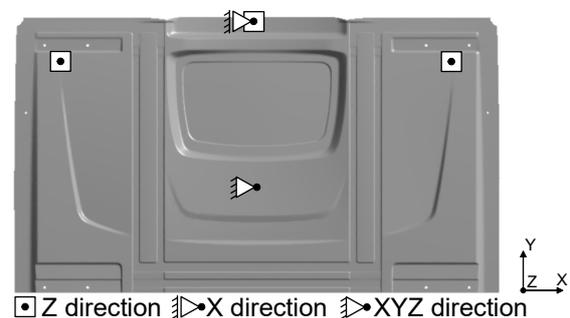
**Figure 2.** Boundary conditions to fix translational and rotational degrees of freedom during simulation.
