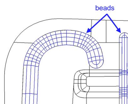
**Figure 10.** Adjusted CAD-model of the truck rear panel for reduction of membrane springback.
