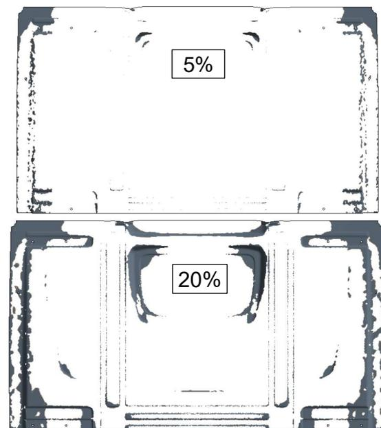
**Figure 6.** Design proposal for the truck rear panel for reduction of membrane springback based on topology optimization.
