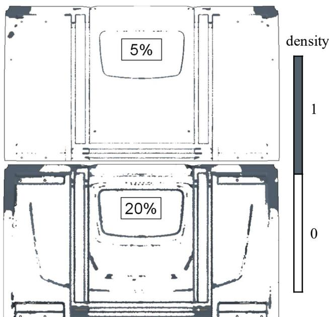
**Figure 5.** Design proposal for the truck rear panel for reduction of bending springback based on topology optimization.
