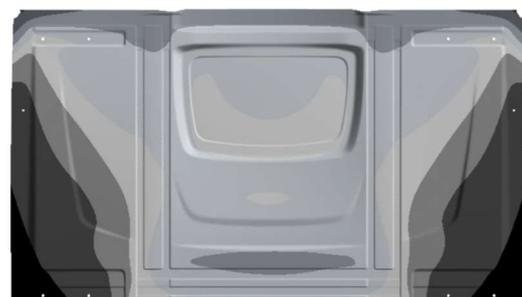
**Figure 4.** Truck rear panel with the calculated membrane springback.
