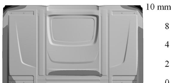
**Figure 1.** Truck rear panel with the calculated springback of the base simulation [5].
