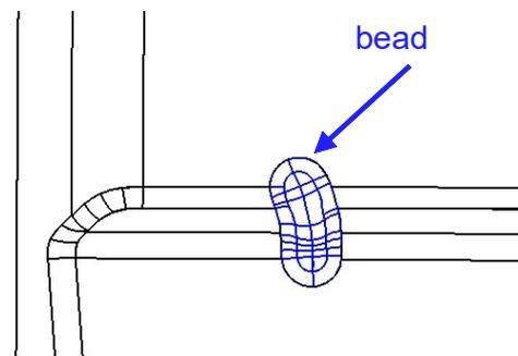
**Figure 8.** Adjusted CAD-model of the truck rear panel for reduction of bending springback.
