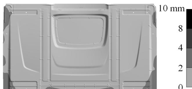
**Figure 12.** Truck rear panel with the calculated springback based on the optimized geometry.
