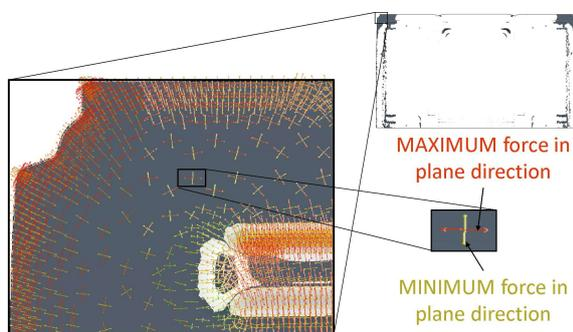
**Figure 9.** *Principle In-Plane Force Dir* from *AutoForm* within the resulting design proposal.
