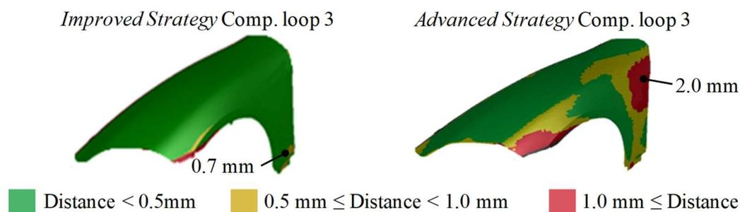
**Figure 8.** Part position in the first flanging operation (*F40*) after three compensation loops
