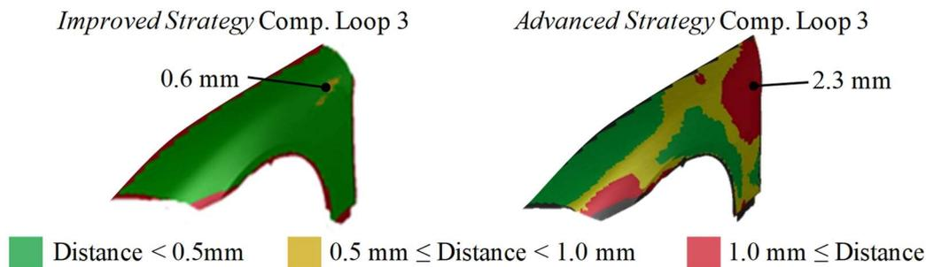
**Figure 9.** Part position in the second flanging operation (*F50*) after three compensation loops
