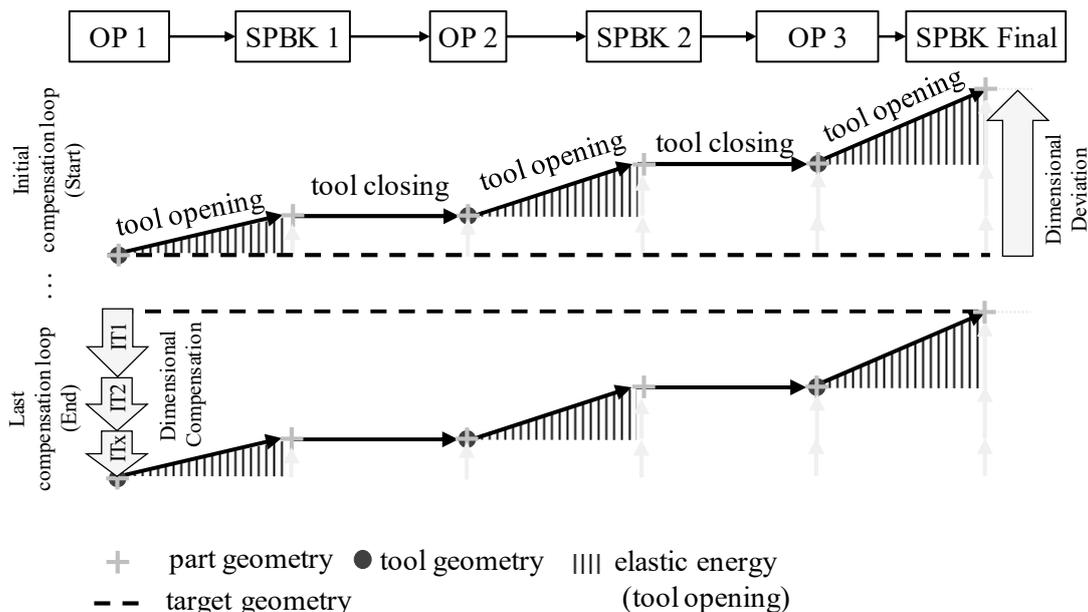
**Figure 2.** Qualitative representation of the dimensional deviations when applying the *Improved Springback Compensation Strategy*
