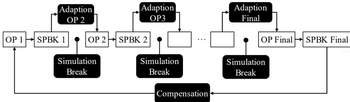
**Figure 1.** Alternating process of adaption and simulation when applying the *Improved Springback Compensation Strategy*
