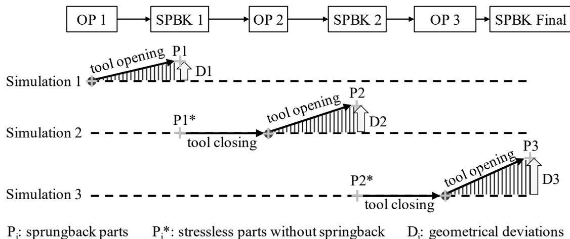
**Figure 3.** Simulation setups and theoretical results by applying the first iteration of the *Advanced Springback Compensation Strategy*
