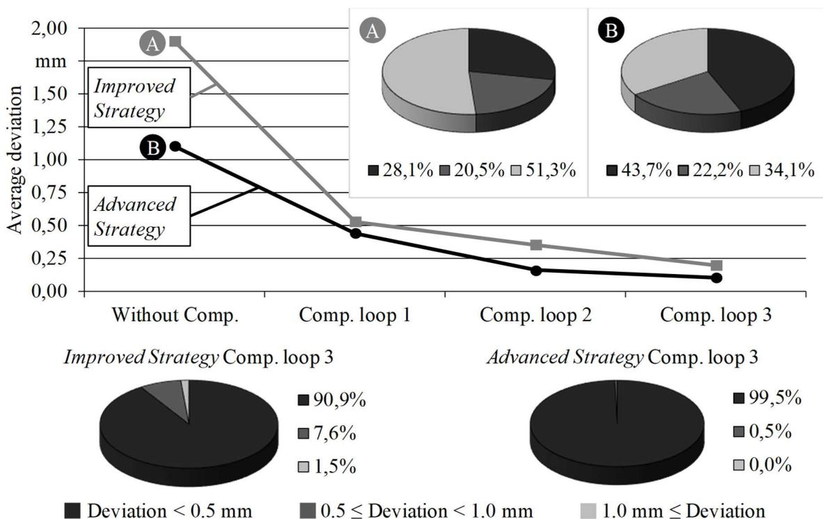
**Figure 10.** Dimensional deviations in the compensation process by using the two different strategies
