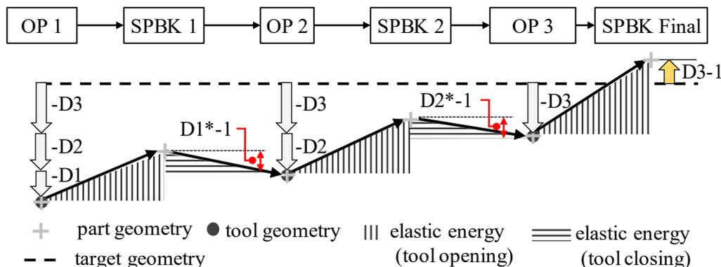
**Figure 5.** Theoretical situation after the first compensation loop by applying the *Advanced Springback Compensation Strategy* (if springback is affected by compensation)
