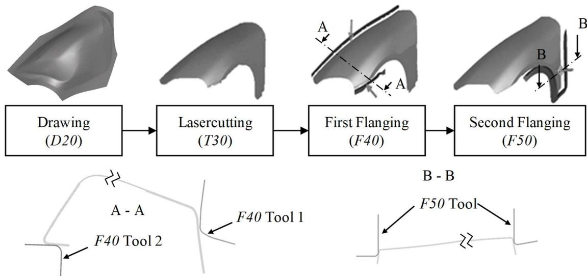
**Figure 7.** Manufacturing process of the aluminium fender
