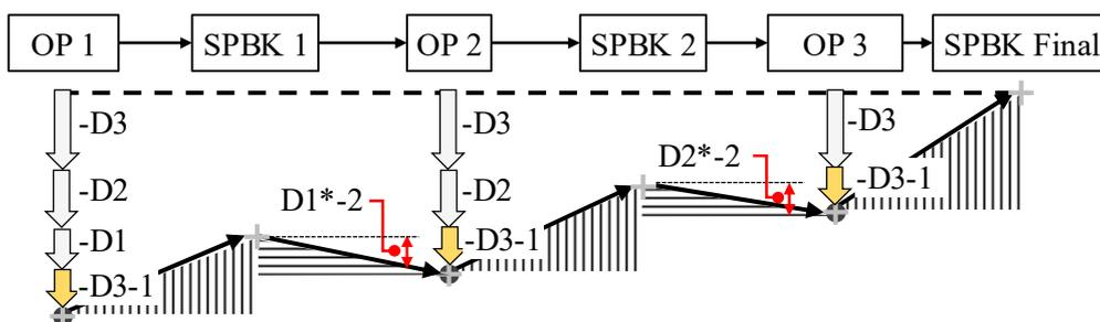
**Figure 6.** Theoretical situation after the second compensation loop by applying the *Advanced Springback Compensation Strategy* (dimensional deviations after OP 3 in tolerance)
