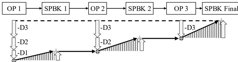
**Figure 4.** Theoretical situation after the first compensation loop by applying the *Advanced Springback Compensation Strategy* (if springback is not affected by compensation)
